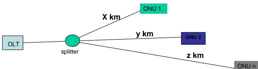
Figure 3: ONUs with different Distances to the Splitter
