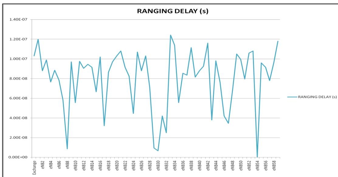
Figure 4.5: Ranging delay for eNBs in the PON network
